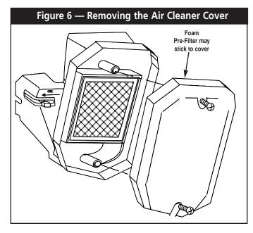
2. Remove the paper air filter and the foam pre-filter from the air cleaner cover (Figure 7).
